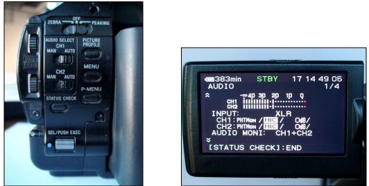
Push in "STATUS CHECK" to see audio levels and if Phantom Power is on
